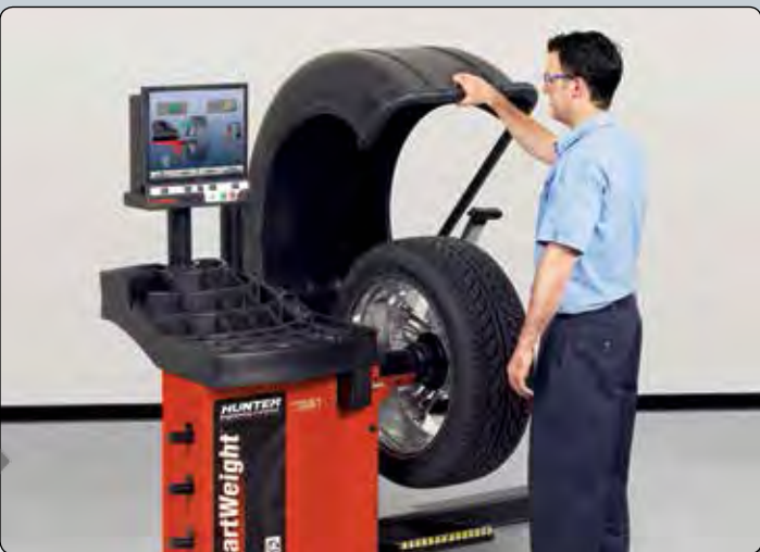
Technician installs weights and performs check-spin
