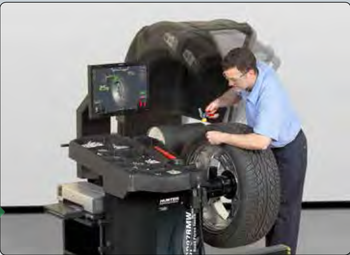
Technician installs weights and performs check-spin
